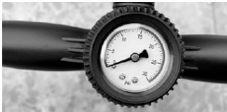
**STEP 6:** Use a pump with gauge, inflate the kite to the recommended 6 psi.
