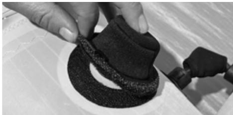
**STEP 7:** Remove the hose from the valve and tighten up the cap by turning it clockwise to the closed position and close the neopren cover.
