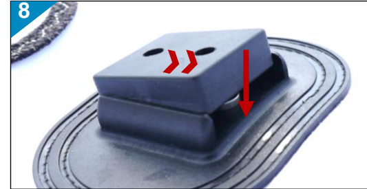
8 Attach the boom-spacer at both outer attachment points. The arrows on the spacers must face each other!
